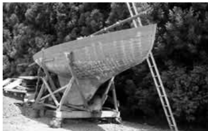
Niobe , (1900, Bailey & Lowe) at the Rescue Trust's yard. The two top planks are coming off
