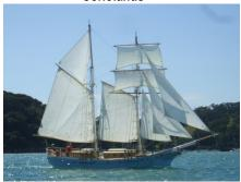
Miniature topsail schooner. Length on deck 24ft, beam 8ft, draft 3ft. Model of a typical ship 4-5 times the length 120 years ago, a work of art with carved figurehead and trail boards. A delight to sail, handy on the helm and stands up well to her canvas, also a viable small cruiser with 3 berths, wood-burning stove with oven, sink, portable toilet, pop-top for headroom. 10hp Bukh diesel suits her well. \$7,500. Contact Bernard Rhodes, (09)372 5621 e.bernard.rhodes@gmail.com
